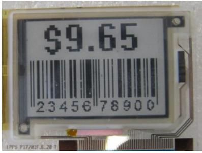
**Figure 2.** Completed ESL Display
