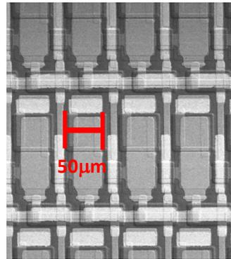
**Picture 5:** SEM Micrograph of an Active Matrix TFT array
