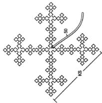
**Figure 3:** Representative concept of Fractal Antennae
