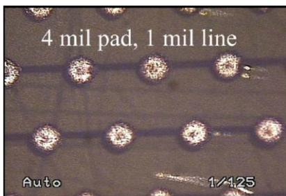
**Picture 3:** Shown are 4 mil pads with 2 mil vias being connected by 1 mil lines.
