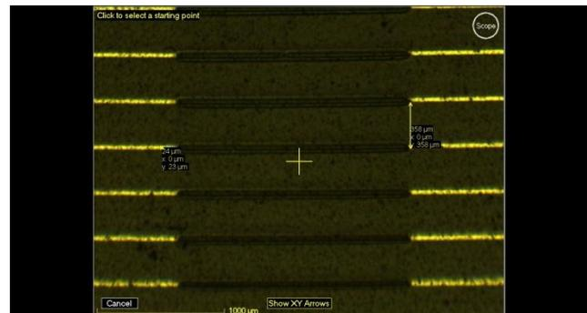
**Picture 9:** 1 mil wide resistors embedded into 1 mil line
