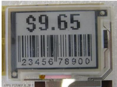
**Picture 6:** Completed Prototype ESL Display
