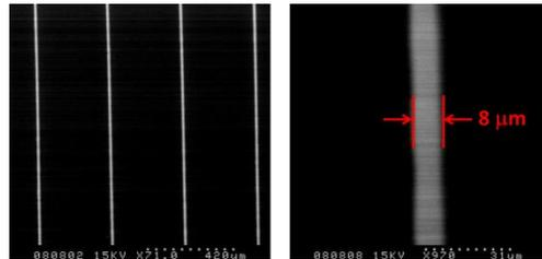
**Picture 4:** SEM micrographs of 8 micron traces this process.
