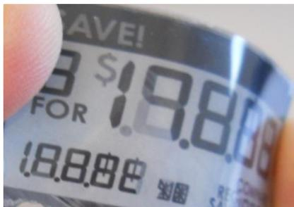
**Picture 7:** Prototype flexible ESL display
