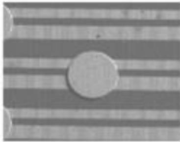
**Picture 2:** SEM micrograph of 10 mil pad with 70 micron and 100 micron trace lines with 50 micron spaces.
