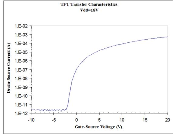
**Figure 2:** Representative Transfer Curve
